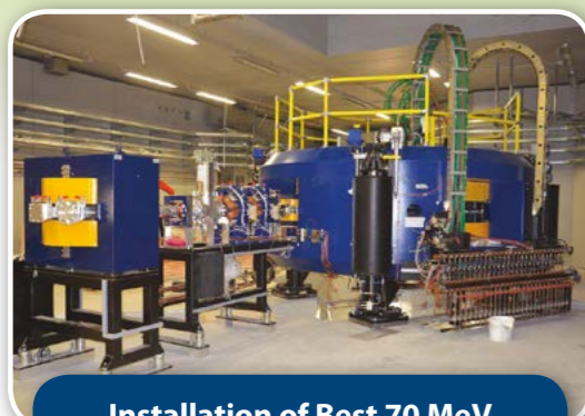
Installation of Best 70 MeV Cyclotron at Italian National Laboratories (INFN), Legnaro, IT
