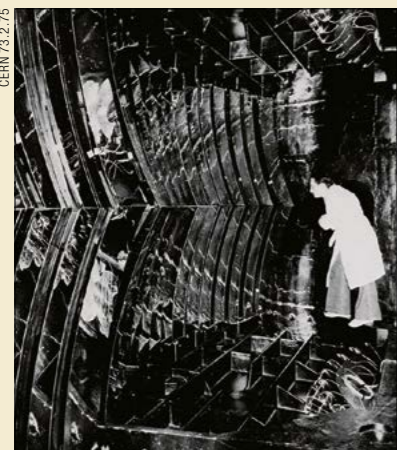
Elliptical mirrors of the large Cherenkov counter used in association with the Omega spectrometer. These mirrors reflect the Cherenkov light onto four sets of parabolic light collectors (sets are visible above and below the white-coated gentleman). The counter, which was built at Saclay, has been working in the CERN West Hall for two years and will also be involved in the first experiments with the 400 GeV proton synchrotron. Meanwhile, it is the essential component of the triggering system in an experiment looking for charmed particles.
