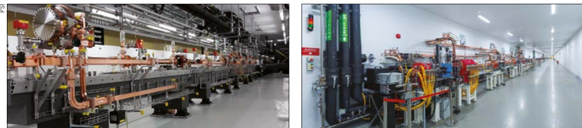
Fig. 3. The SwissFEL C-band linac at the Paul Scherrer Institute (left) and the injection linac for the SINAP XFEL test facility at the Shanghai Institute of Applied Physics (right). Both projects work closely with CLIC to advance high-gradient RF technology.
